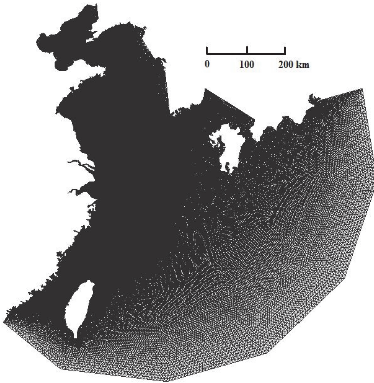
Fig. 6. A sketch of triangular grid for modeling typhoon-induced storm tide
